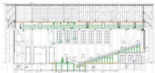
Main Section - from left: stage area, fixed floor, modular floor with orchestra pit, manual seating riser system, capacity extension on first floor
